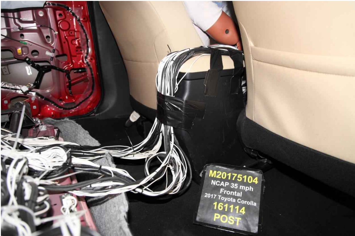
029 Post-Test Dummy Cable Routing
