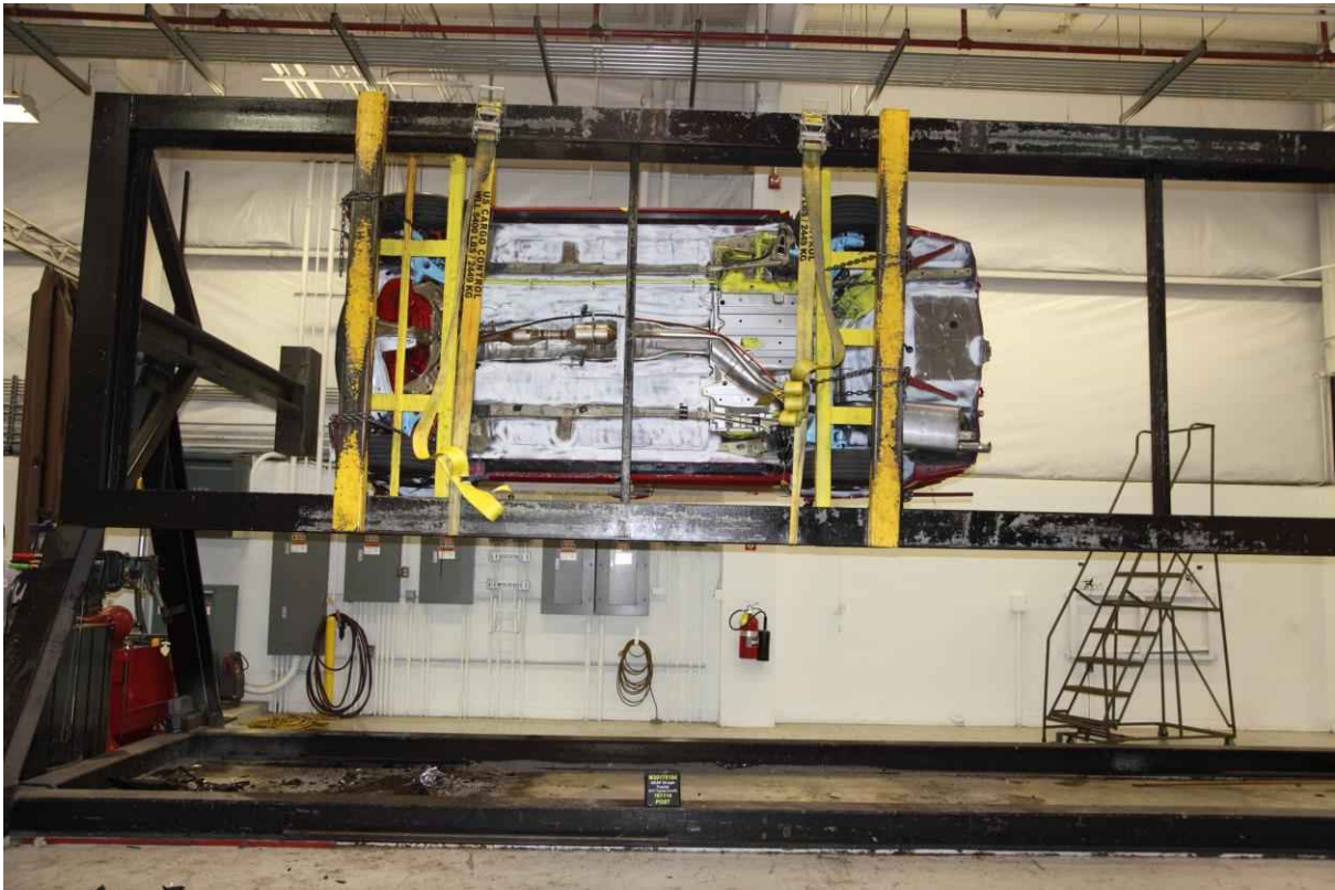
076 Vehicle at 270° on Static Rollover Device
