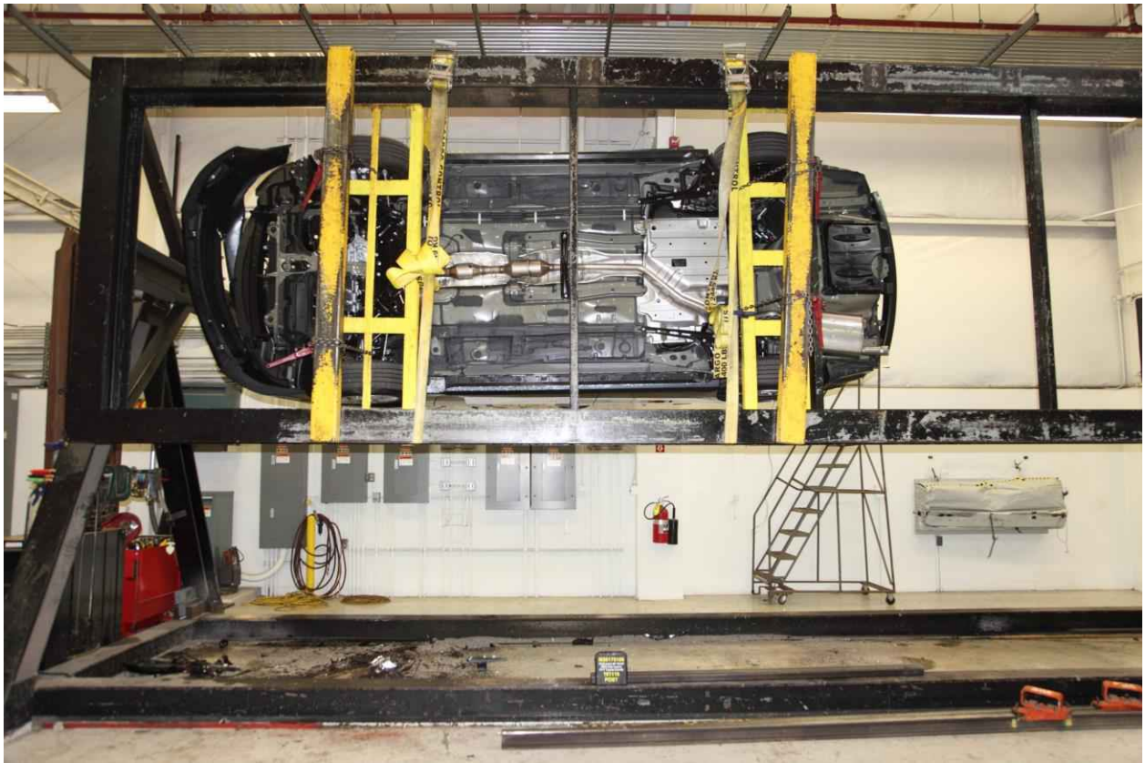
099 FMVSS No. 301 Static Rollover 270 Degrees
