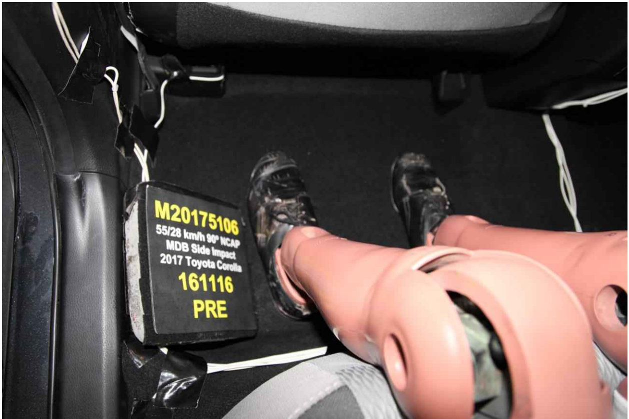
064 Pre-Test Placement of Rear Passenger Dummy Feet
