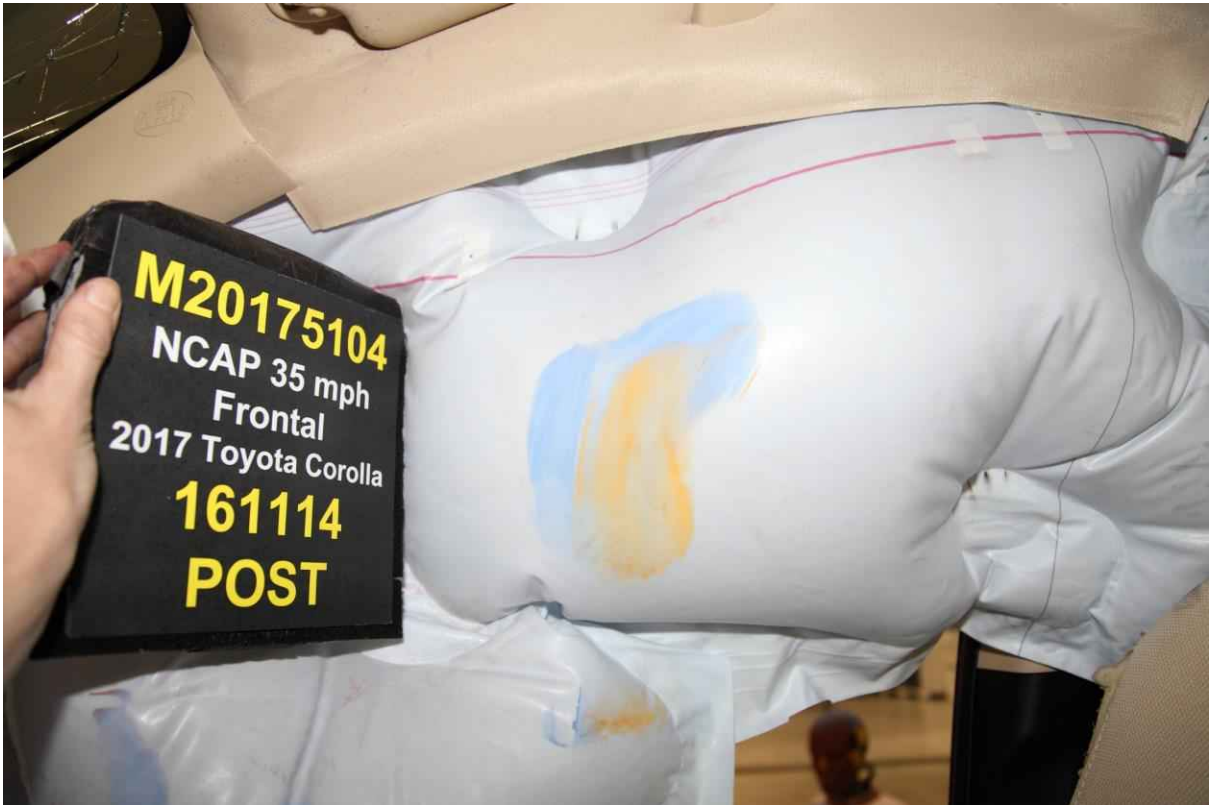
069a Post Test Passenger Dummy Contact with Side Curtain Airbag
