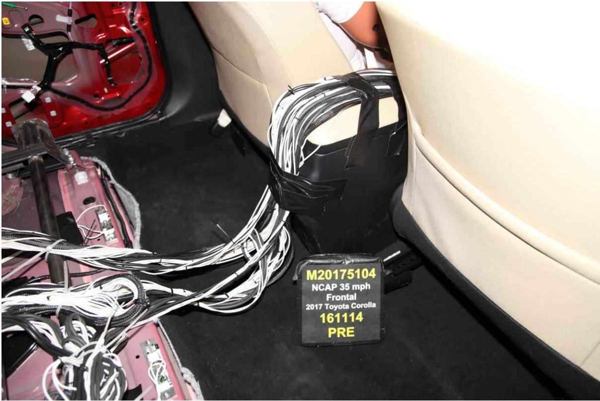
028 Pre-Test Dummy Cable Routing
