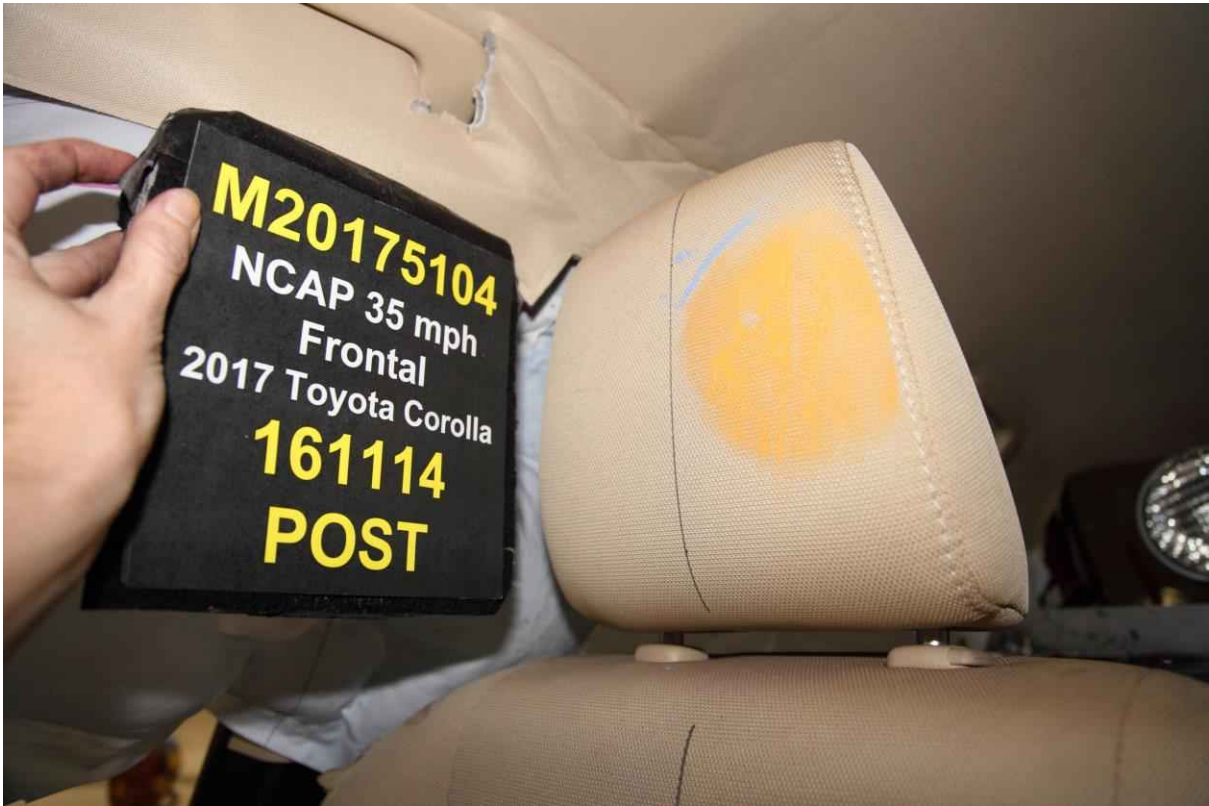
069 Post Test Passenger Dummy Contact with Headrest
