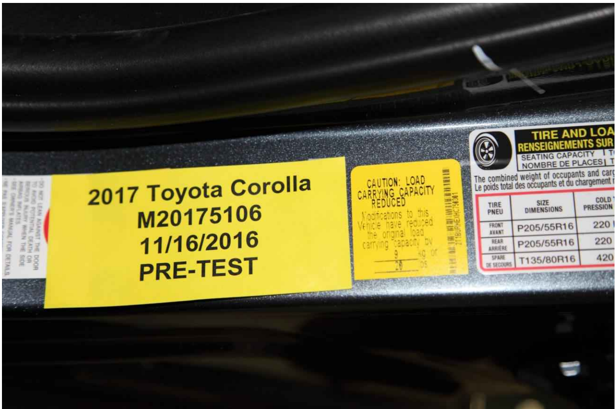
092a Close-Up View of Reduced Load Capacity Label
