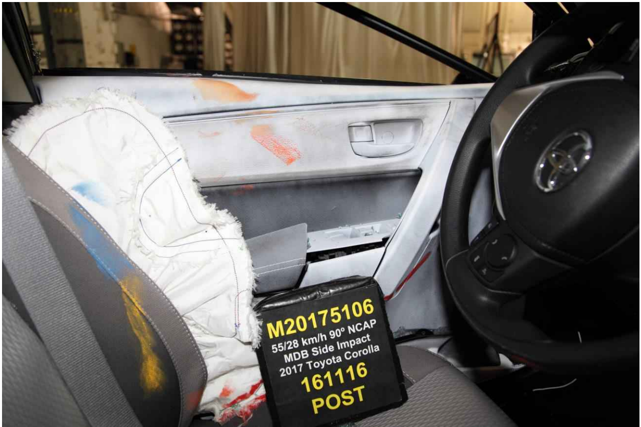
050 Post-Test Driver Dummy Close-Up Torso Contact with Vehicle Interior View
