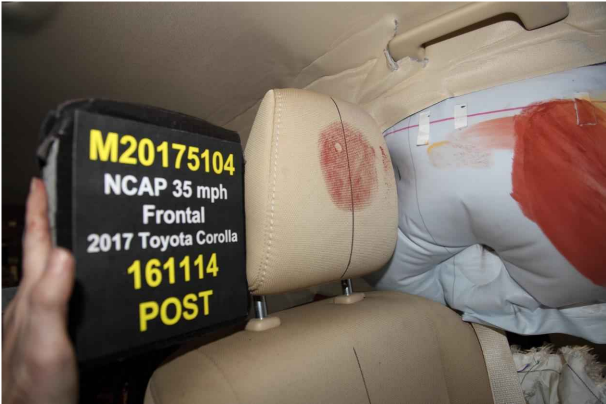
048 Post-Test Driver Dummy Contact with Headrest
