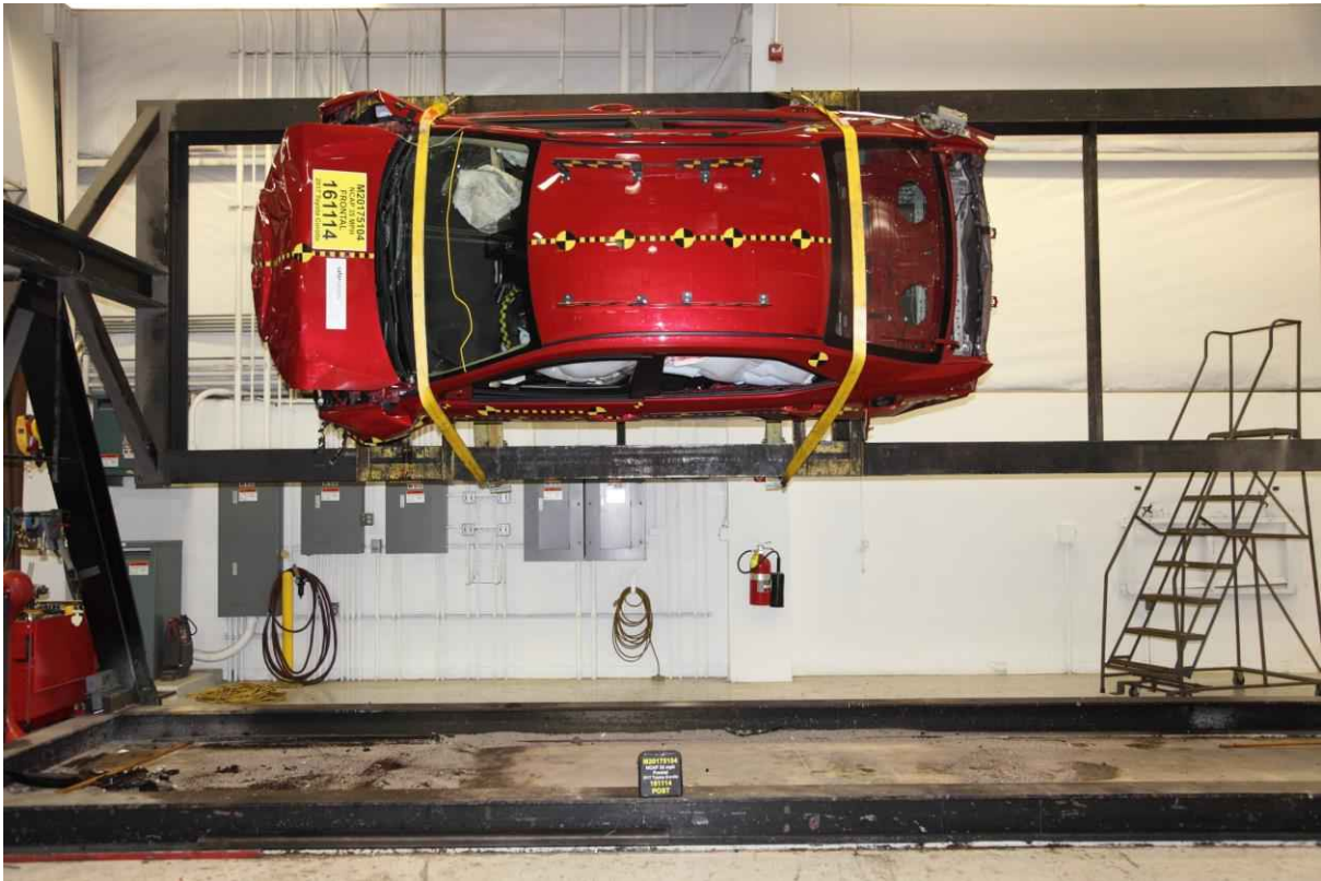
074 Vehicle at 90° on Static Rollover Device
