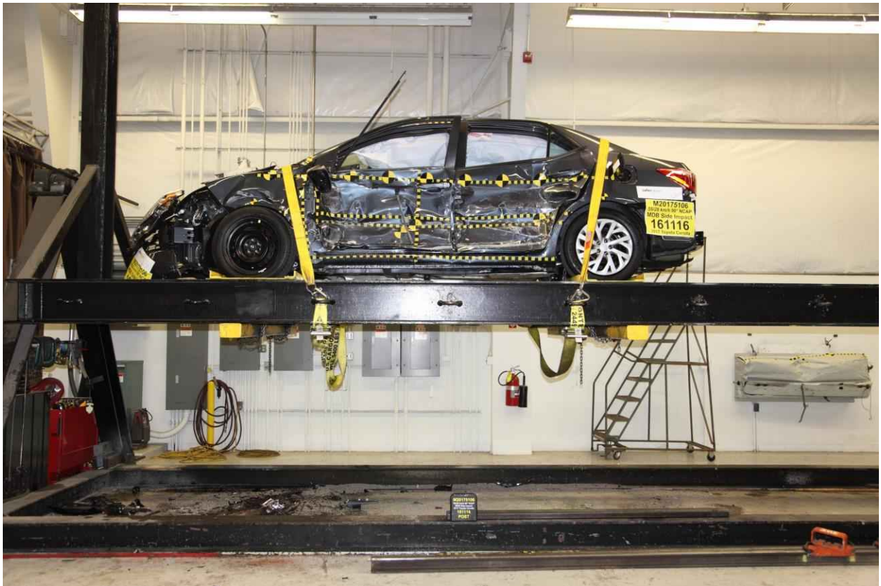
100 FMVSS No. 301 Static Rollover 360 Degrees
