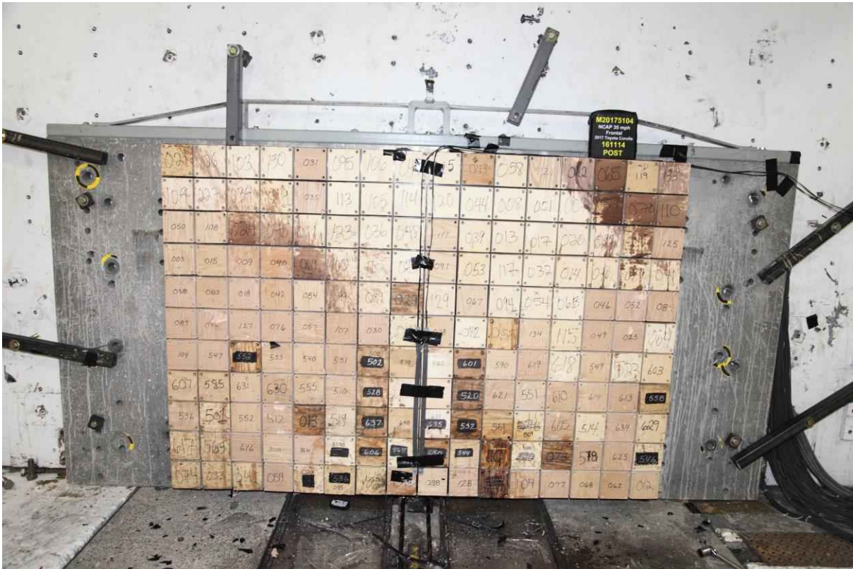
003 Post-Test Load Cell Wall
