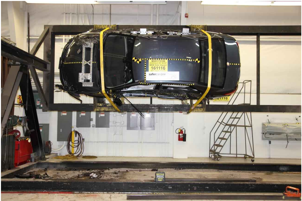
097 FMVSS No. 301 Static Rollover 90 Degrees
