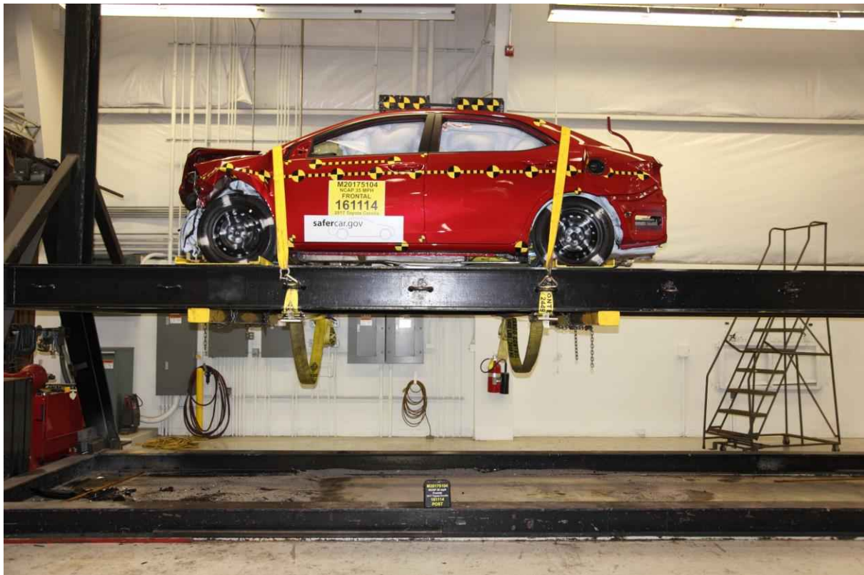
073 Vehicle at 0° on Static Rollover Device
