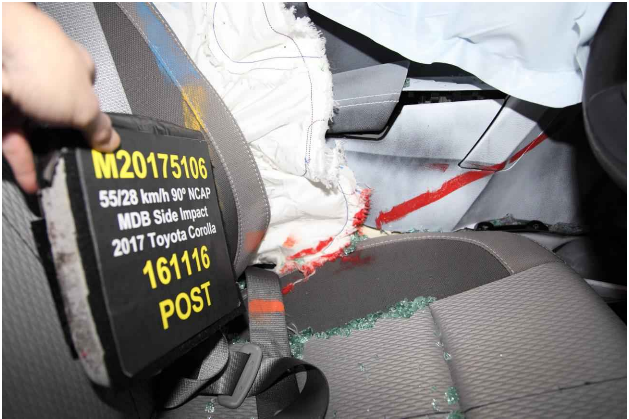
052 Post-Test Driver Dummy Close-Up Pelvis Contact View
