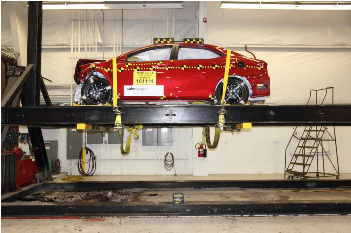
077 Vehicle at 360° on Static Rollover Device
