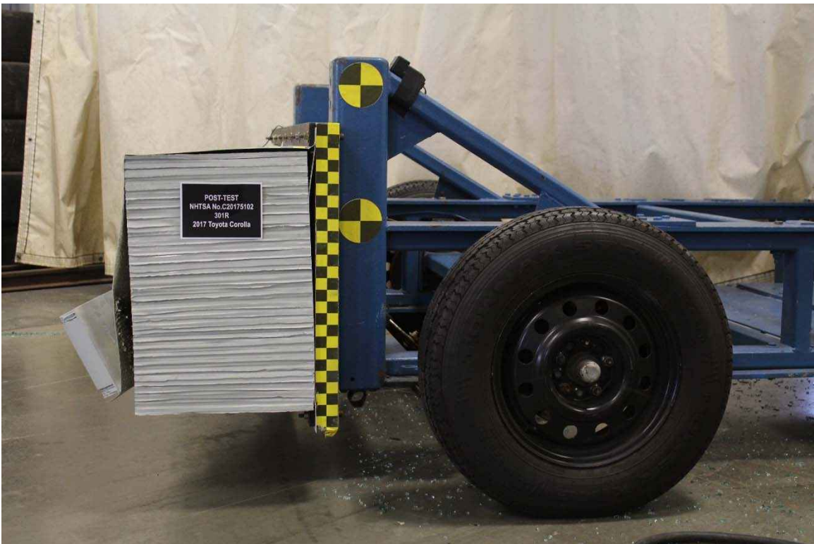
Figure A-22: Post-Test MDB Left Side View
