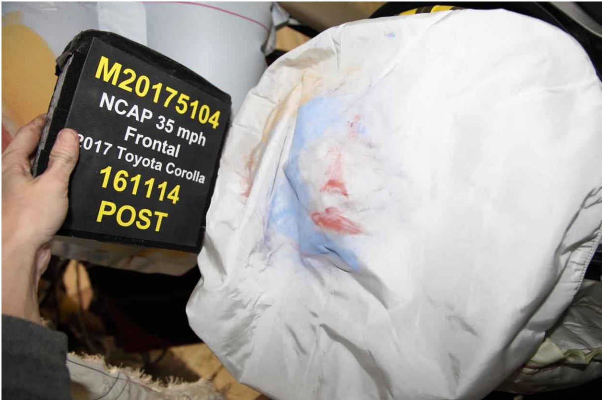
047 Post-Test Driver Dummy Contact with Airbag
