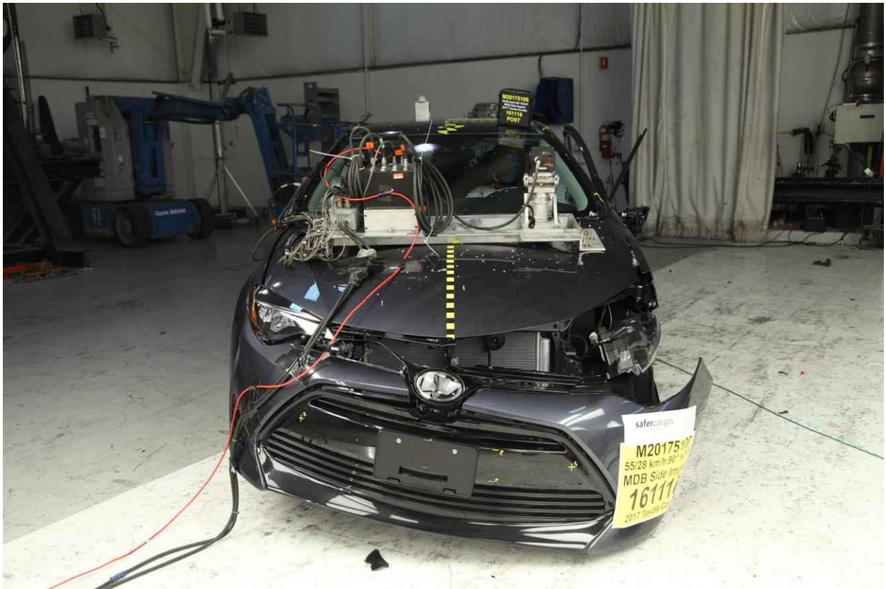
004 Post-Test Frontal View of Test Vehicle
